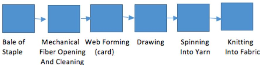
As you can see from the diagrams, producing nonwoven fabrics has fewer steps than woven or knit fabrics. Also, the production speed for making staple fiber nonwoven fabrics is much faster (100 to 400 yards per minute) than woven fabrics (0.5 to 6 yards per minute) and knit fabrics (2 to 16 yards per minute). Because of the higher speeds and reduction of steps, nonwoven fabrics cost much less to produce.
